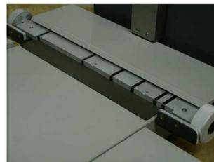
Original way of positioning design, perfectly meets the needs of various sizes photobook mounting by using two sets magnetic positioning piece (different thickness) and a steel ruler.
