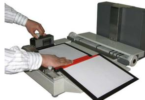
Can measure the spine, position the block in the center of the cover and clamp the cover. With the flexible and extendable platform, it is convenient to mount large size of cover.
